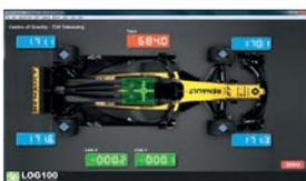
The Center of Gravity (CoG) function found within LOG100 gives you the tools to quickly calculate and visualize center of gravity from up to eight sources of weight data. Choose your weight data, specify the X and Y coordinates and let the LOG100 do the work to calculate and display the position of CoG.
