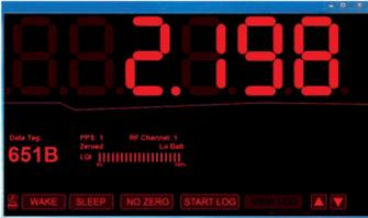
This software allows you to quickly detect, pair, view and log data from a load cell device. System requirements: Windows 10,8 and 7 with USB base station
