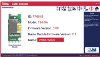
This software allows you to quickly and easily configure, test communication and calibrate wireless load cell devices. System requirements: Windows 10,8 and 7 with USB base station.
